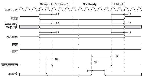
† <u>XBE[3:0]/XA[</u>5:2] operates as address signals XA[<u>5:2]</u> during expansion bus asynchronous peripheral accesses.
