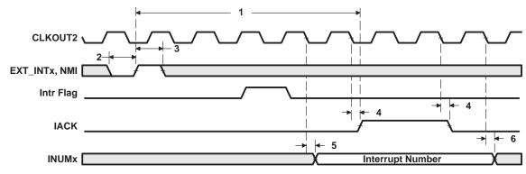
Figure 27. Interrupt Timing
