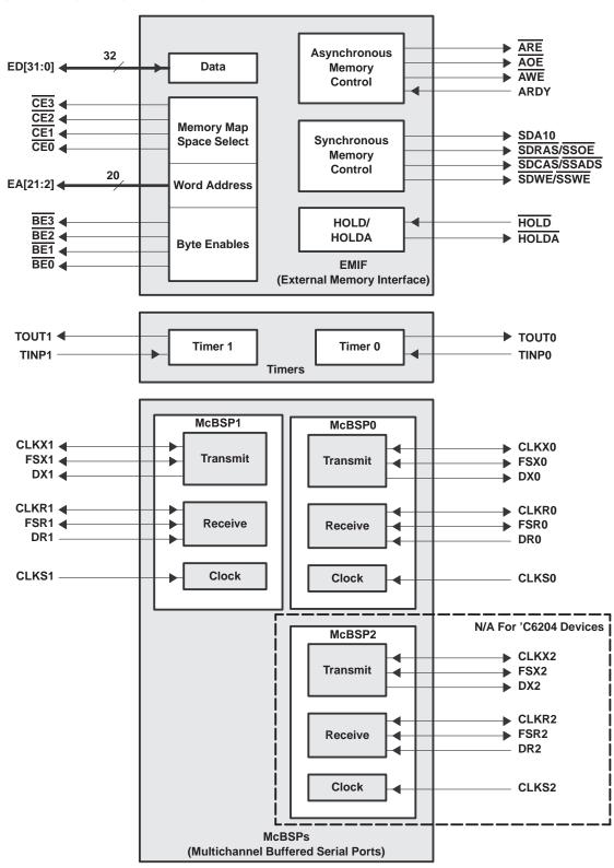
Figure 3. Peripheral Signals
