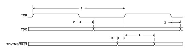
Figure 53. JTAG Test-Port Timing
