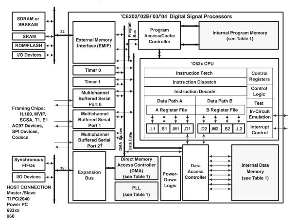
functional and CPU block diagram ('C62x devices)
