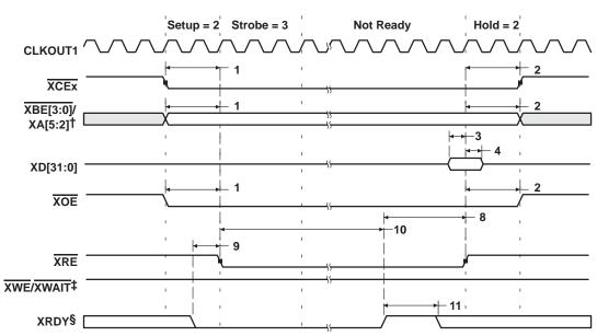
TXBE[3:0]/XA[5:2] operates as address signals XA[5:2] during expansion bus asynchronous peripheral accesses.
