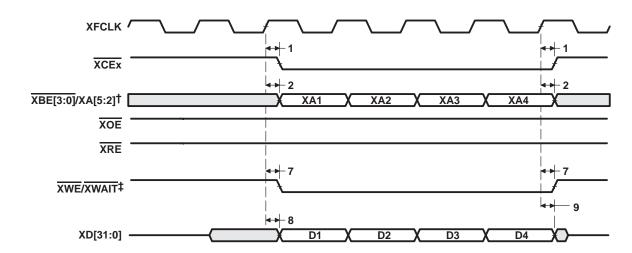
TBE[3:0]/XA[5:2] operates as address signals XA[5:2] during synchronous FIFO accesses.
