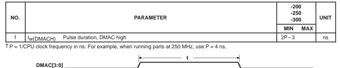
Figure 50. DMAC Timing
