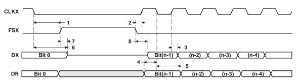
Figure 46. McBSP Timing as SPI Master or Slave: CLKSTP = 10b, CLKXP = 0
