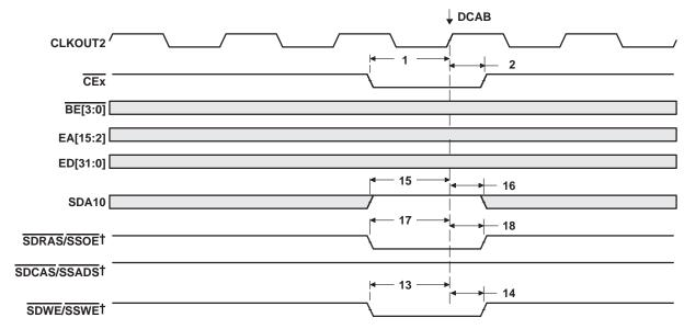
† SDCAS/SSADS, SDRAS/SSOE, and SDWE/SSWE operate as SDCAS, SDRAS, and SDWE, respectively, during SDRAM accesses.
