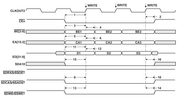
T SDCAS/SSADS, SDRAS/SSOE, and SDWE/SSWE operate as SDCAS, SDRAS, and SDWE, respectively, during SDRAM accesses.
